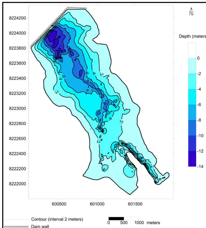
Figure 3. Bathymetric map of Chisoba reservoir.
