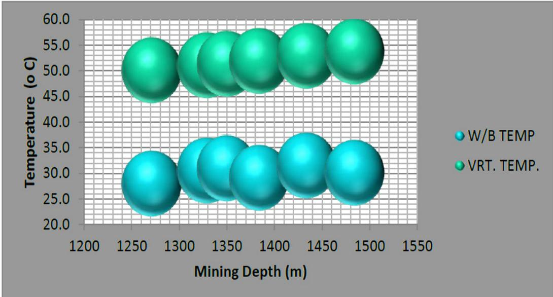
**Figure 12:** Virgin Rock Temperature as measured on a linear scale against depth of mining
