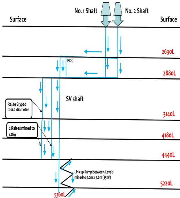
**Figure 5:** Current Downcast Ventilation System
