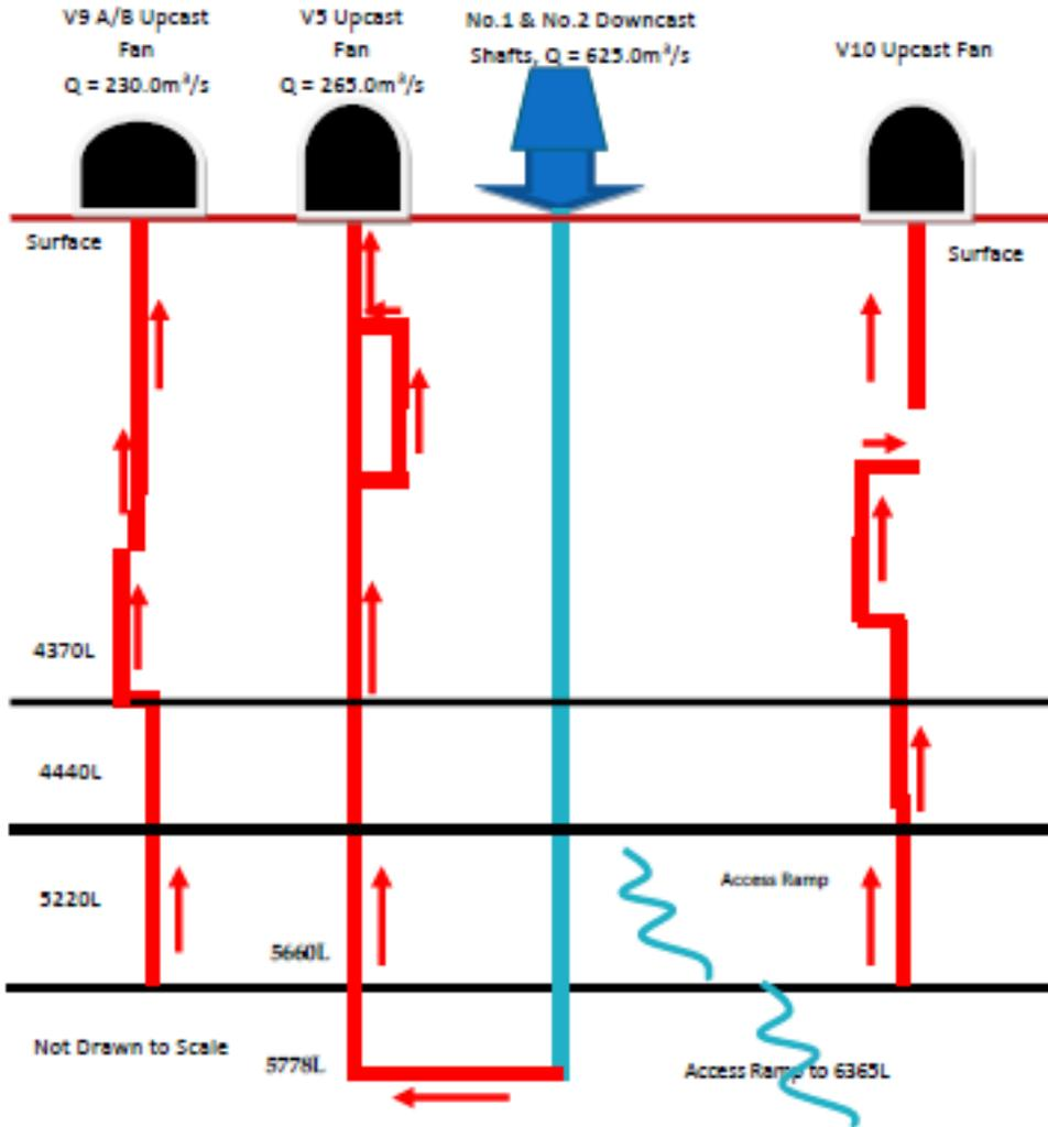
Figure 6: Current Upcast Ventilation System
