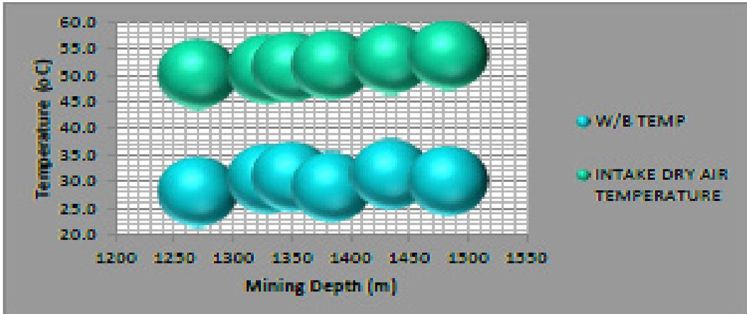
**Figure 13:** Intake Dry air Temperature/Wet-bulb Temperature Depth of mining
