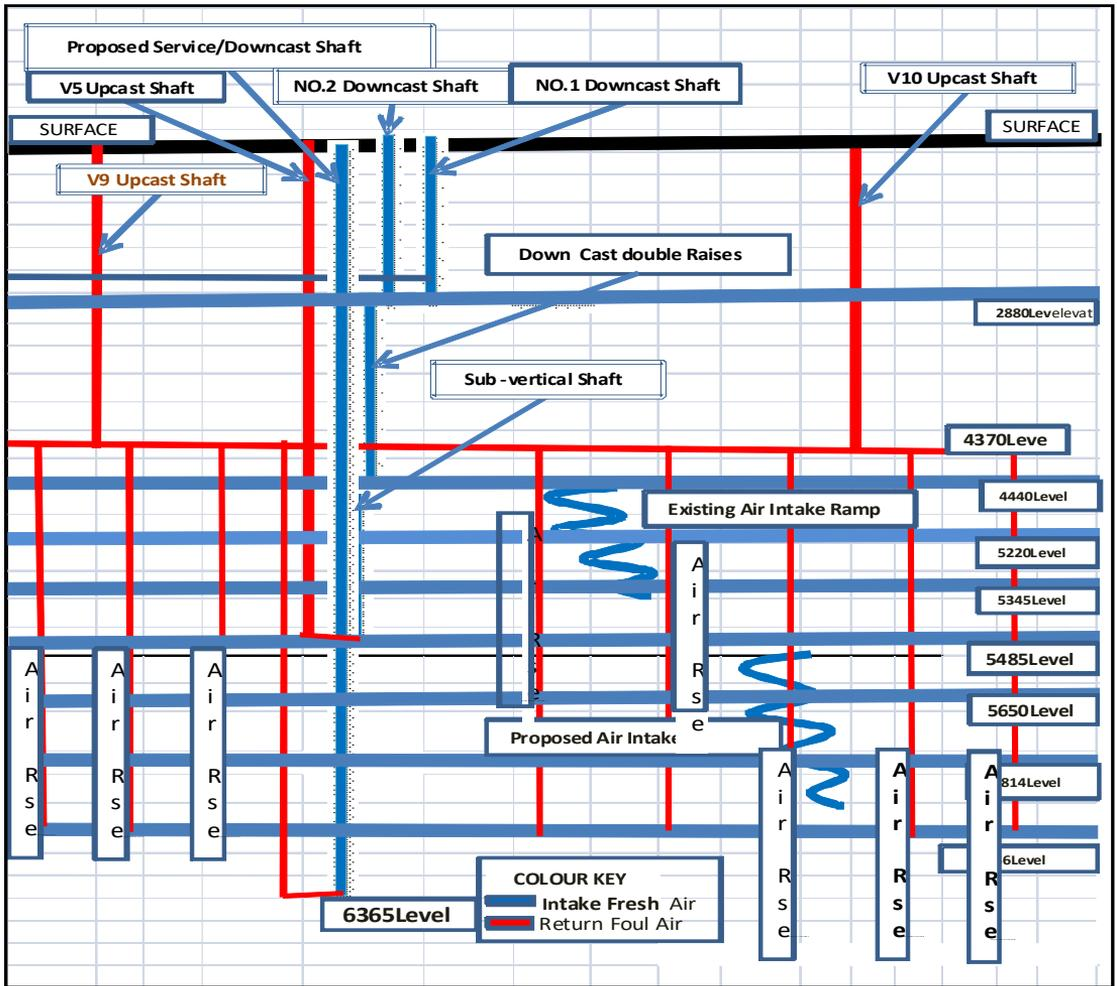
**Figure 14:** Profile of Designed Parametric Data obtained from the computer simulation of mine ventilation network.
