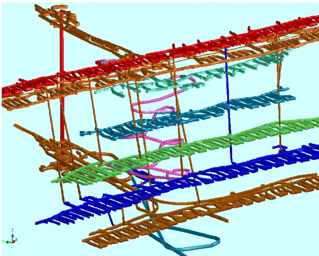
**Figure 2:** Mindola Sub-Vertical Mine General Layout of Mining Method showing VCR chamber excavations (Mopani Copper Mines - Mindola Mine Planning Department, Report, 2014).
