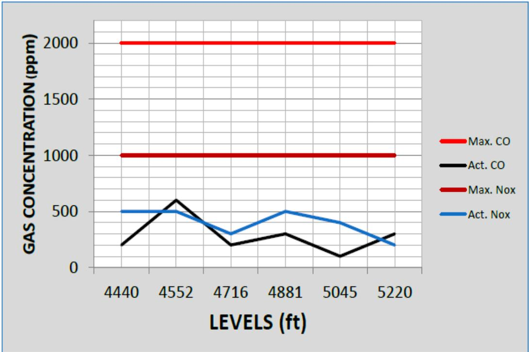
Figure 9: Diesel Equipment Exhaust Gas Concentrations vs Legal Limits
