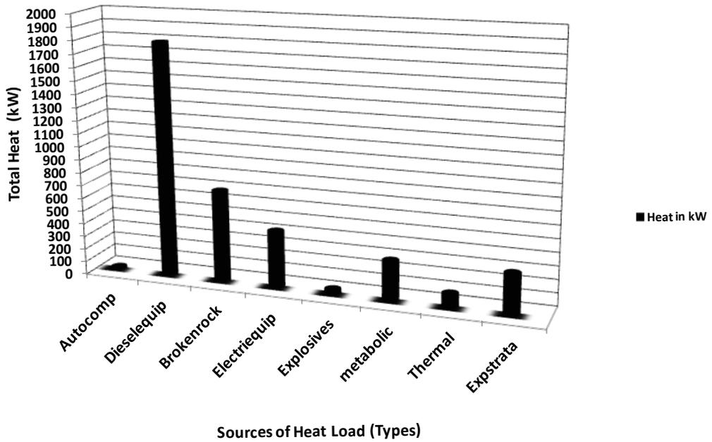
Figure 11: TOTAL HEAT LOADS FROM VARIOUS SOURCES (4440L – 5220L Ore Zone)
