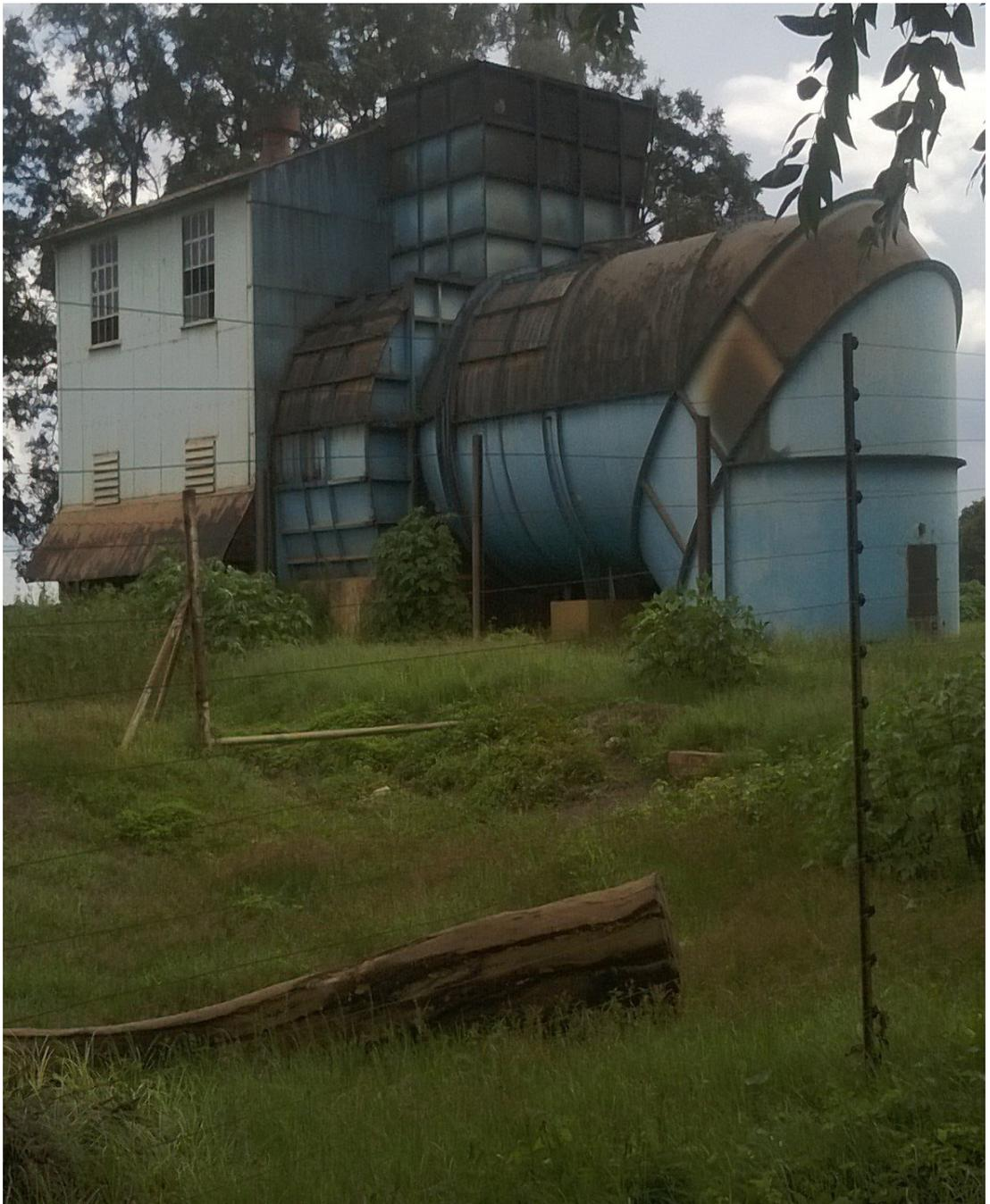
**Figure 7:** V10 Upcast Main Fan Mindola Mine-A typical Upcast fan
