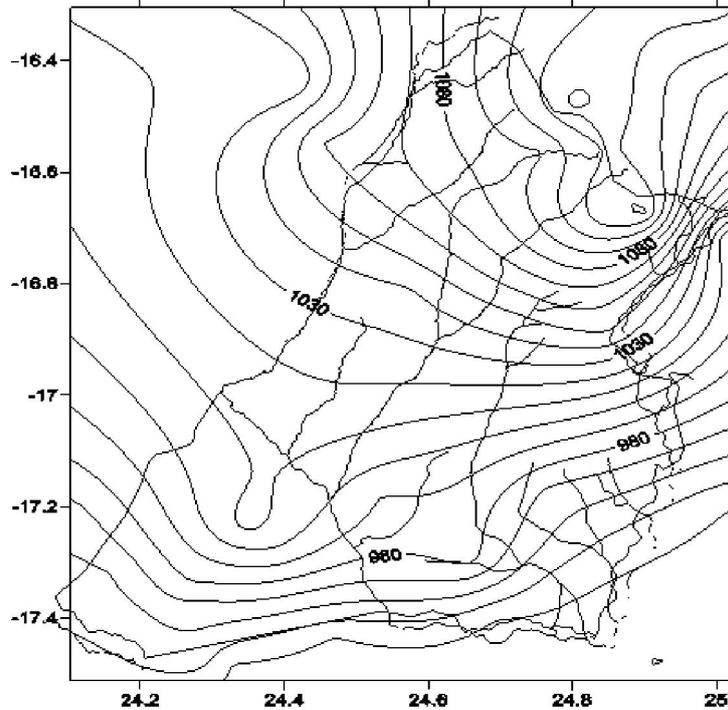
Figure 10: Map of Sesheke showing the measured hydraulic gradient indicating slightly steeper gradient in the North-west to South East direction.
