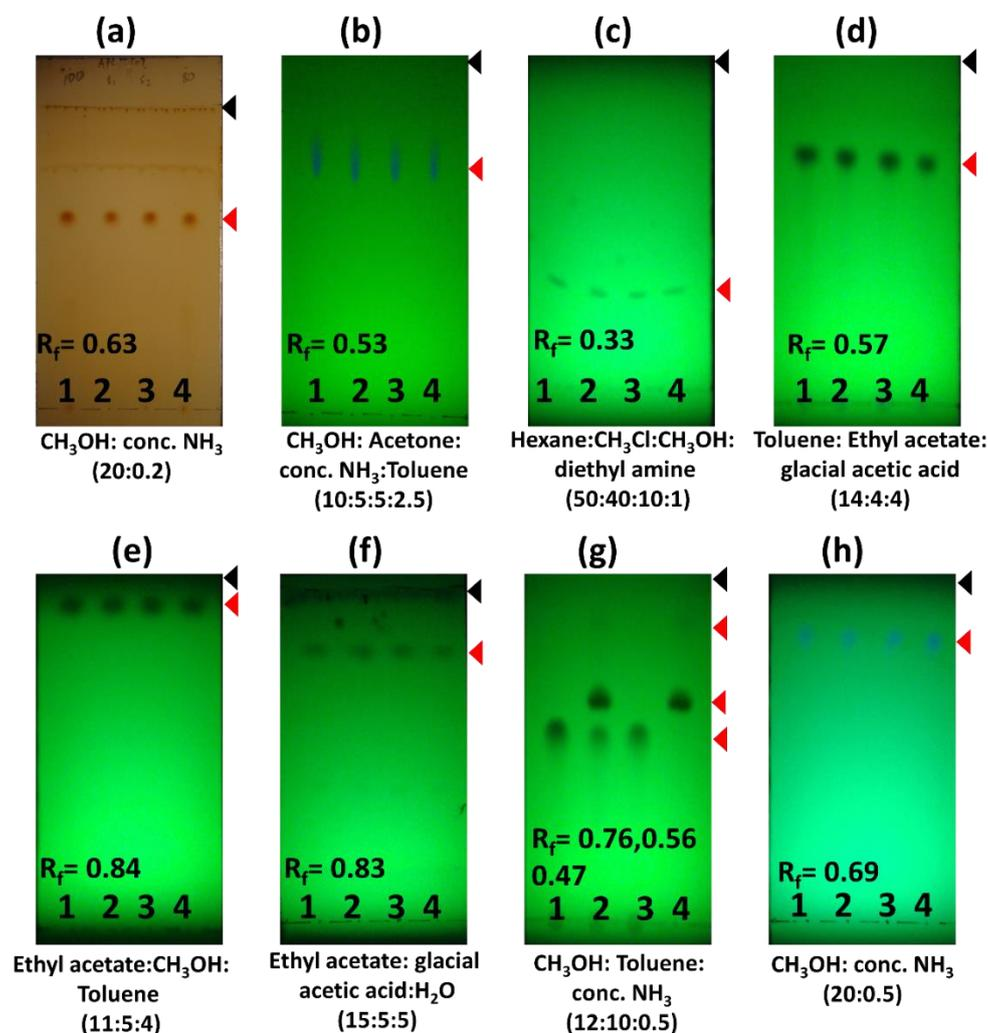
**Figure 1:** Shows the HPTLC F254, Aluminum support, Silica gels irradiated at 254nm UV. Panel **a**;Atenolol-100 mg, **b**; Ciprofloxacin-500 mg, **c**; Ketoconazole-2%, **d**;Mebendazole-500 mg, **e**;Nevirapine-600 mg, **f**;Penicillin V-250 mg, **g**;Rifamate (Isoniazid-75 mg. Rifampicin-150 mg combination),**h**;Quinine sulfate-300 mg.
