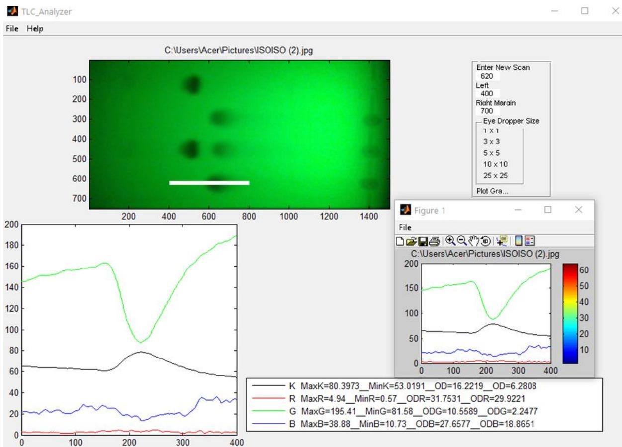
**Figure 3:** Typical image and intensity results of DeTLC. The figure shows lane 1 of the isoniazid standard at 100%.
